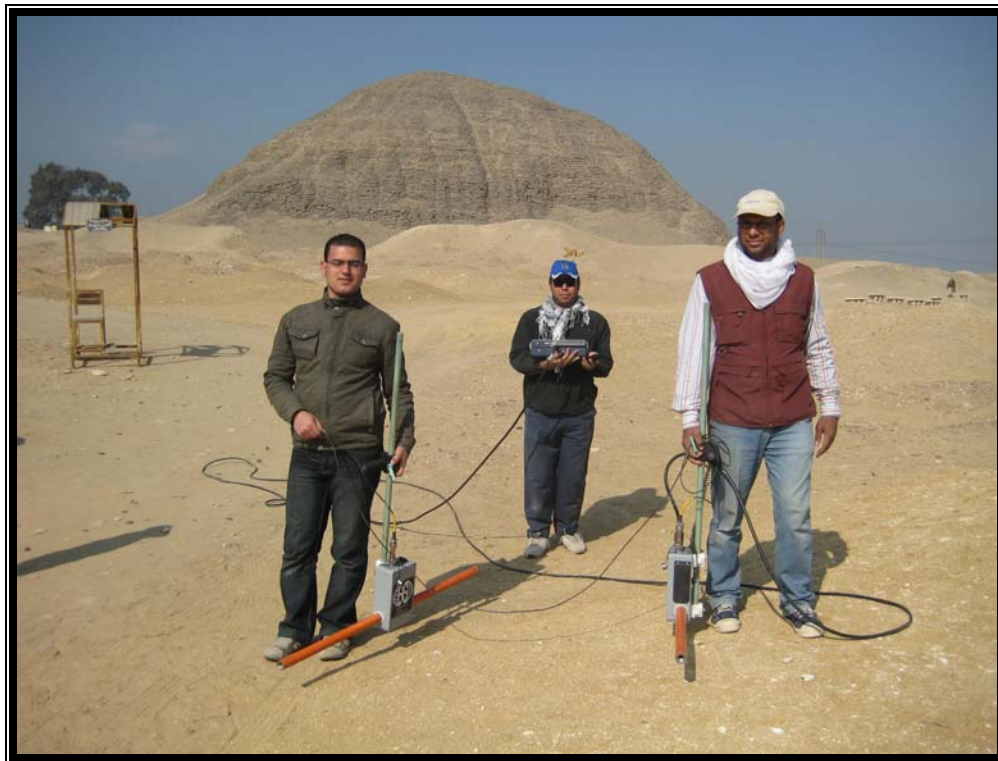
Fig. (7): Ground penetrating radar survey at Hawara area.
