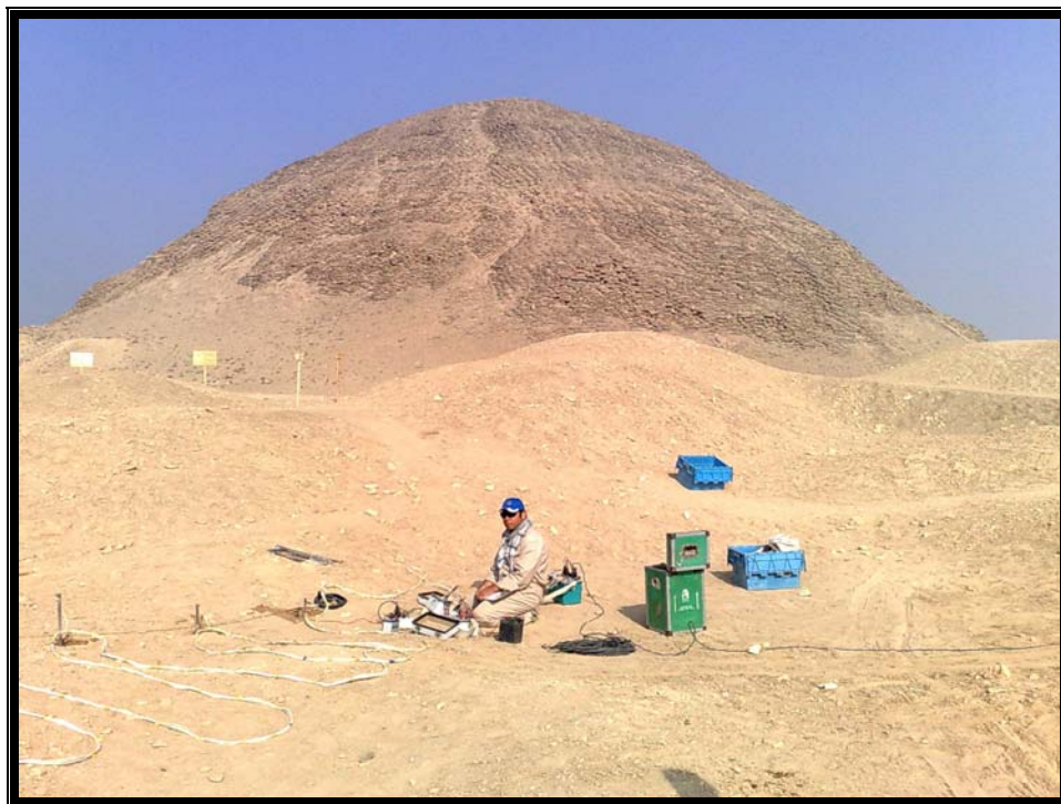
Fig. (5): Electrical resistivity tomography at Hawara area.
